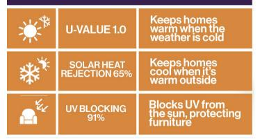
\*Based on a unit construction of 4mm custom ambient toughened/ 16mm argon filled cavity/ 4mm clear toughened
